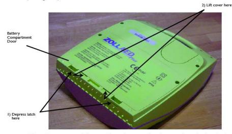
2. Remove all batteries at once and dispose of batteries properly. Place new batteries into the battery bank, observing battery polarity markings and making sure that all batteries are securely seated and properly oriented. After placing the first 5 to 9 batteries in the battery well, the INSTALL BATTERIES audio prompt reminds you to install the remaining batteries in the battery compartment.
